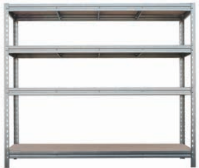
BULLRACK 2XL - 1 mm 200x210x60 cm Levels: 4 Loading per level: 600 kg Finish: GALVA RAL 7016
